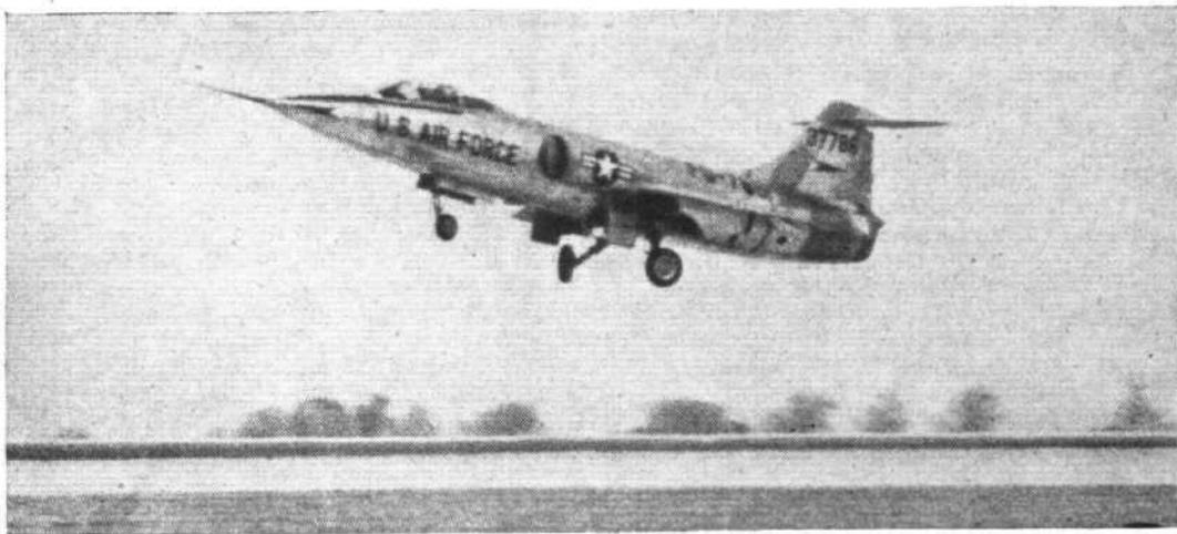
Landing, the same aircraft—one of the J65 Sapphire-powered prototypes—streams its braking parachute to ease the wear and tear on the Bendix multi-disc brakes.
