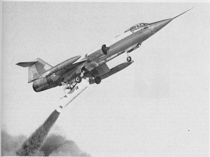
The F-104 in the "Zell" configuration for a zero length takeoff.
